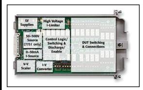
Three source/switch plug-in modules provide the Model 2790 with programmable high voltage and low current sources, connection switching, and signal conditioning circuitry.
