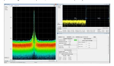
Sophisticated WLAN measurements are easy. On the 802.11g signal shown below, the spectrogram shows the initial pilot sequence followed by the main signal burst. The modulation is automatically detected as 64 QAM for the packet and displayed as a constellation. The data summary indicates an EVM of -33.24 dB RMS, and burst power is measured at 10.35 dBm. SignalVu-PC applications are available for 802.11a/b/j/g/p, 802.11n and 802.11ac to 40 MHz bandwidth.
