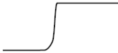
Signal with a short length ground lead
