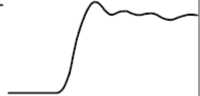
Signal with a long ground lead
