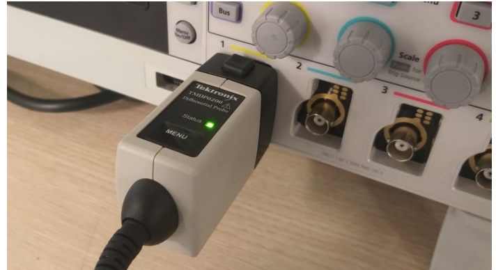
TekVPI probes communicate scale settings, ranges, and status to the TBS2000B.
