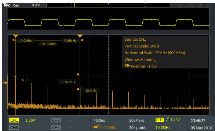
The time domain source waveform can be displayed above the FFT frequency spectrum.
